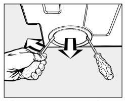
Remove only the cover cap. Do not remove the frame.
